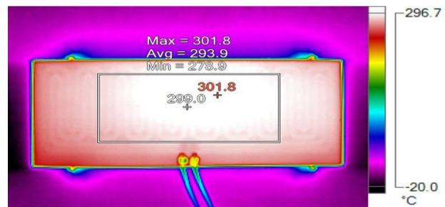
Infrared measured delta temperature front to back surface is in the range of 12°C – 18°C. A thermocouple reading on the back side (plate) states 288°C.
