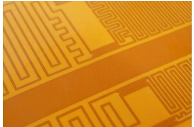
Etched foil heater multiple heat zones.
