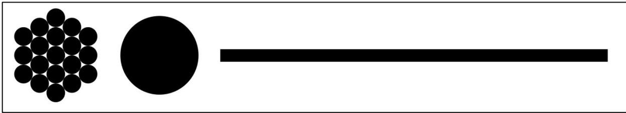
Equivalent cross sectional areas of 19 strand .003" dia wire, solid wire, and .002" thick foil.
