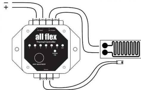
As soon as power is introduced to the unit, the device will present an electronic serial code for 5 seconds. Each of the 7 LEDs will either be ON, OFF, or FLASHING. Note each LED function and record the digital serial code for future reference. The 7 LED serial code represents the temperature setting combination of the temperature settings of the 6 yellow LEDs stored in the controller.
