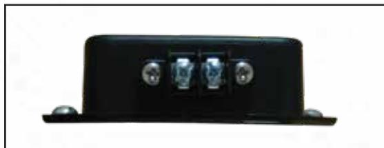
Terminal blocks provide discrete wire screw connection for input power, output power (to heater), and sensor.
