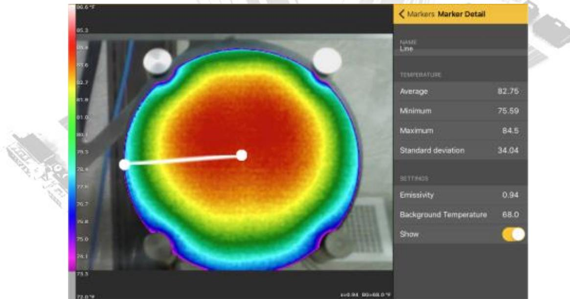
Figure 8: Thermal Image of Uniform Heater after 10 minutes and 5 volts Input Voltage
