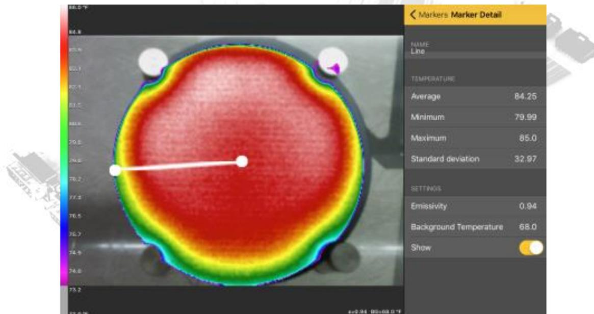
Figure 6: Thermal image of profiled heater after 10 minutes and 5 volts input voltage
