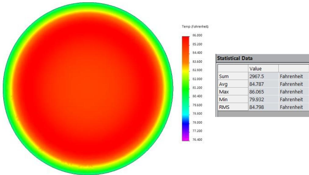
Figure 5: Profiled heater simulation results after 10 minutes and 5 volts input voltage
